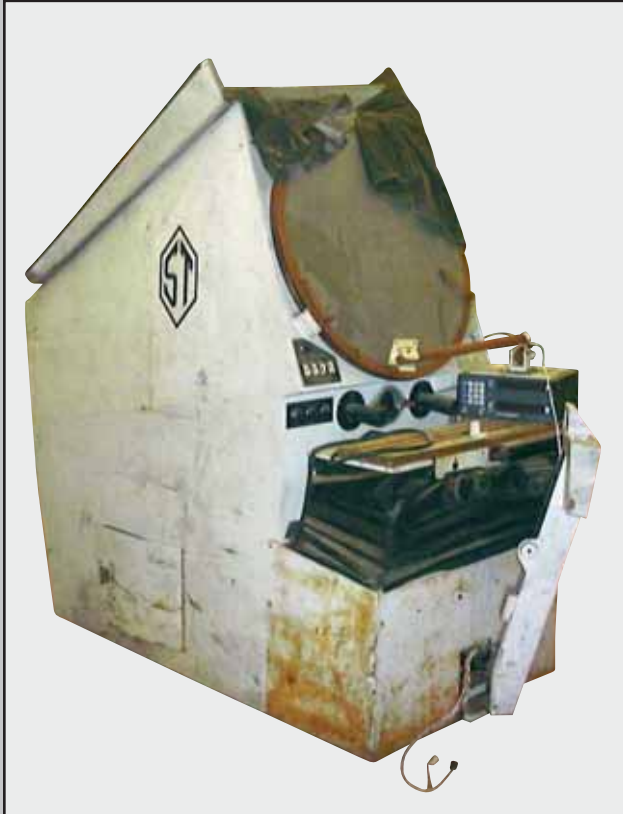
Above: Actual photo of customer's 26 year old 2600 Series 30" Comparator when received at S-T Industries to be remanufactured.
