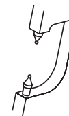
Fixed ball or roll contacts Can be used in conjunction with side stops to check pitch diameter of helical gears
